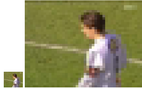
Figure 4: DC image example. Each 8 \times 8 pixel block has one DC value, hence the dimension of the DC image of a 352 \times 288 pixel image is only 44 \times 36 . Enlarged version included for illustration purposes.
